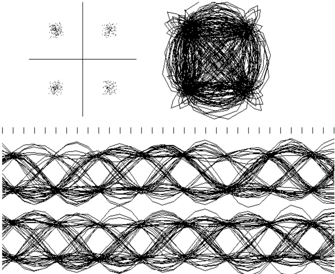
Figure 9 A QPSK Constellation Plot and Eye Diagram of a Signals Distorted with 4.4 dB of Amplitude Tilt over 2.5 MHz. , MER = 18.5 dB
