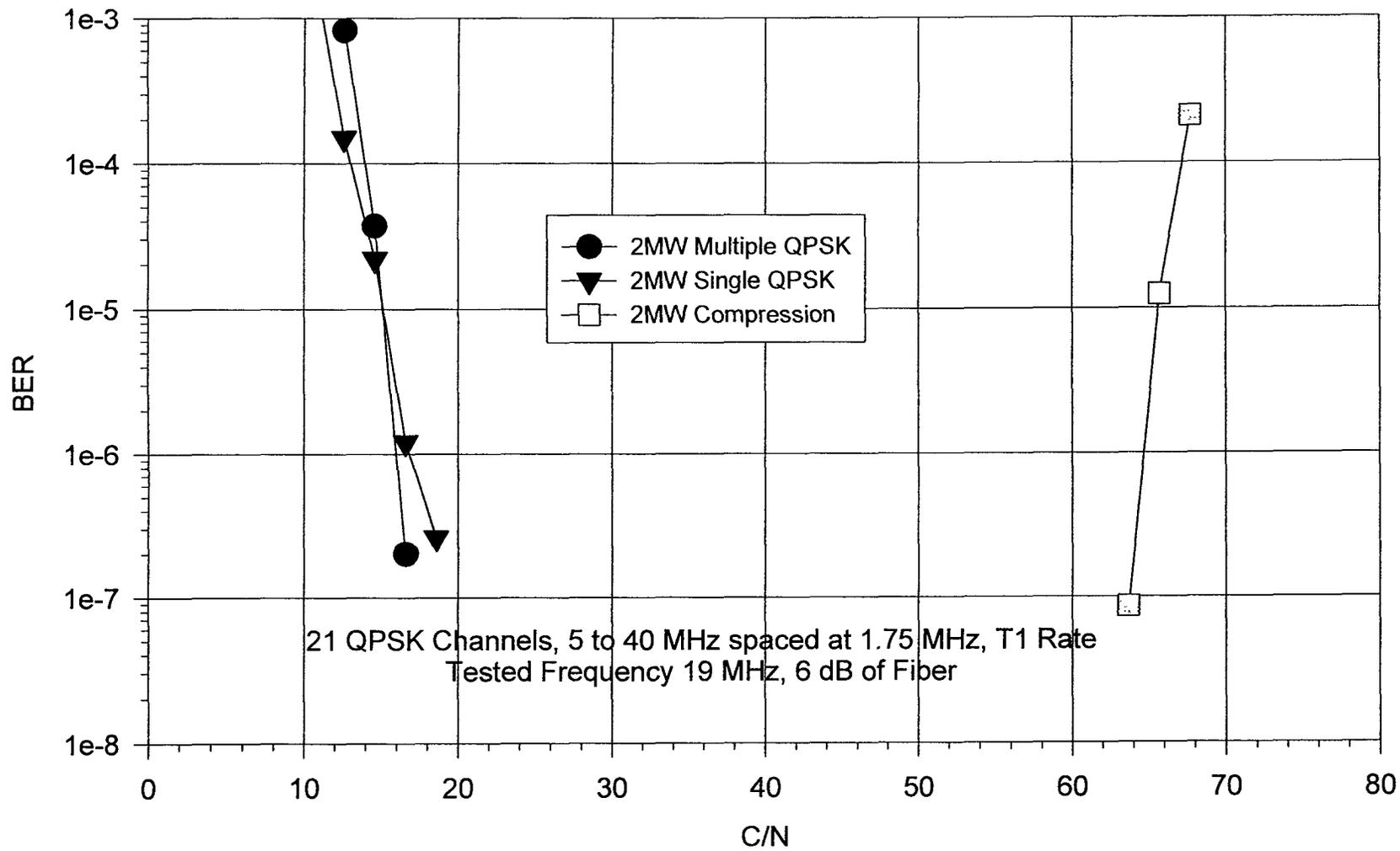
21 QPSK Channels, 5 to 40 MHz spaced at 1.75 MHz, T1 Rate
