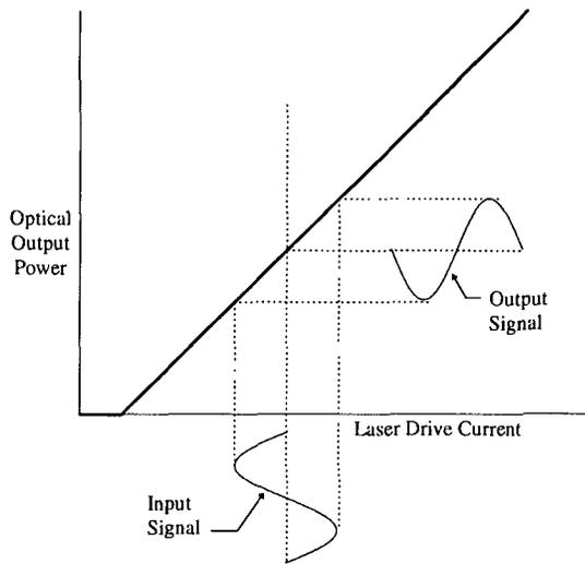
**Figure 2a: Externally-Modulated Signal in Linear Operation**
