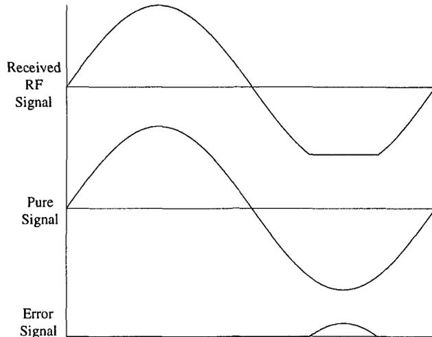
**Figure 4: Decomposition of External-Modulator Clipping**
