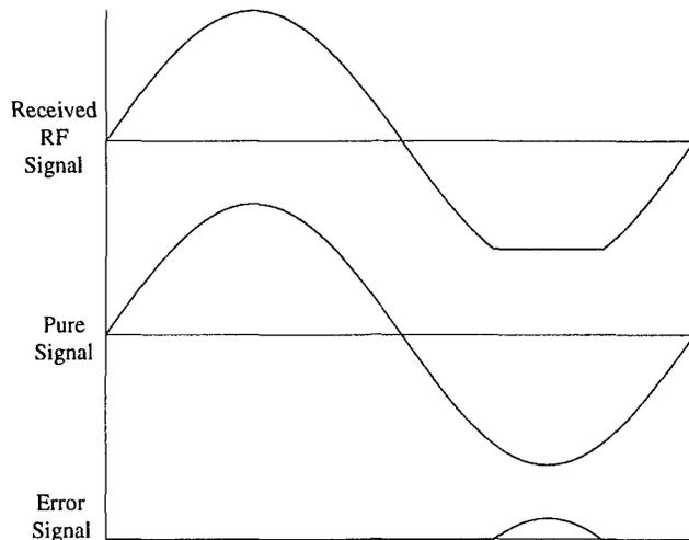
**Figure 4: Decomposition of External-Modulator Clipping**
