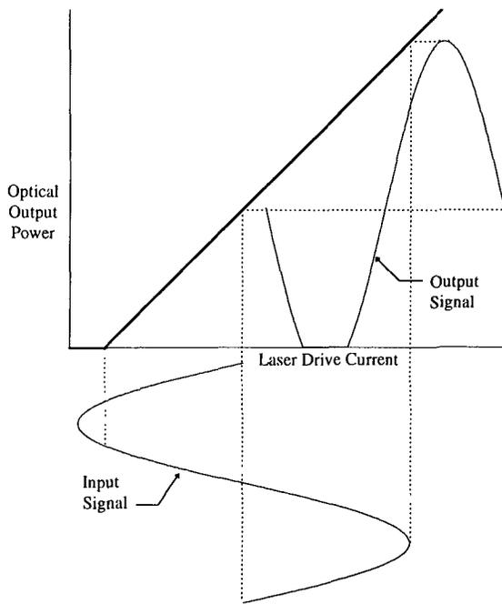
**Figure 2b: Externally-Modulated Signal in Clipping**
