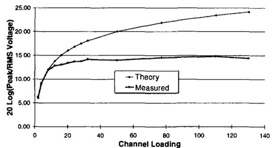
Note that the theory predicts a continuous increase in peak-to-RMS ratio as the number of channels grows. However, the test results indicate that the ratio levels out between 14 and 15 dB. We believe that the reason the peak-to-RMS ratio does not continue to increase as predicted has to do with noise in the system. In particular, the phase noise and frequency stability of the CW generator are likely fluctuating enough to prevent any more precise coherent adding of the carrier phases.
