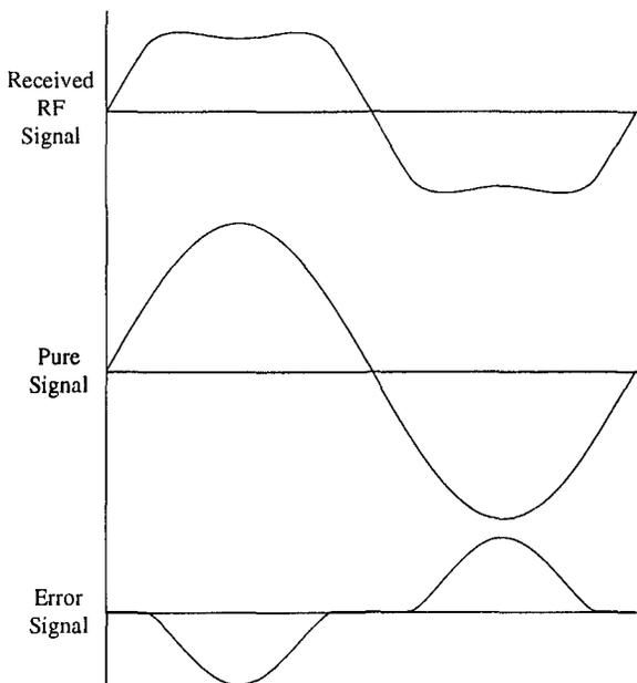
A more critical difference between the clipping effects in these two types of transmitters results from the fact that in DFB's the laser is actually turned off (biased below threshold) when the RF signal gets too large in the negative direction. Unfortunately, the RF optical signal out of the laser does not appear to recover instantaneously.
