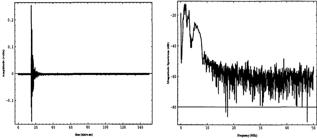
Figure 13. Shielded static electricity discharge time and frequency responses.
