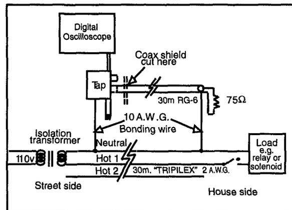
Figure 10. Lab experiment 1 simulating home wiring
