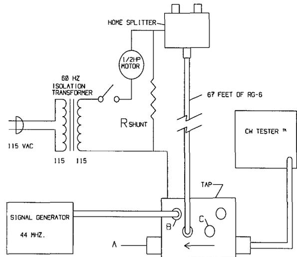
Figure 16. Lab experiment 2 simulating ferrite saturation in the tap.
