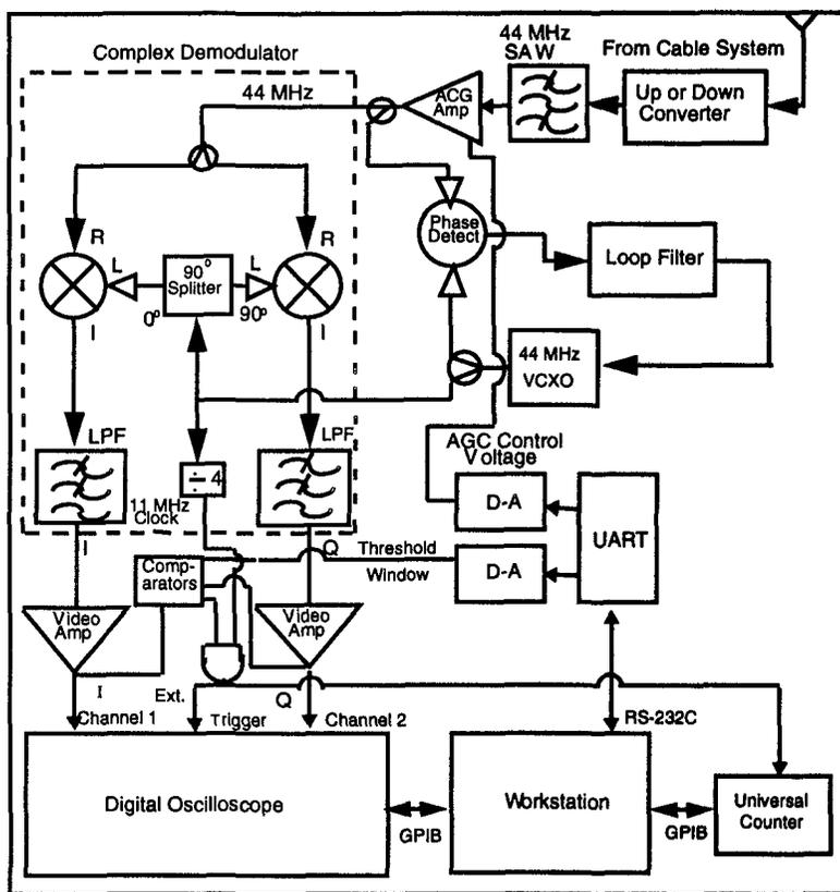
Figure 2. CW Tester™ block diagram
