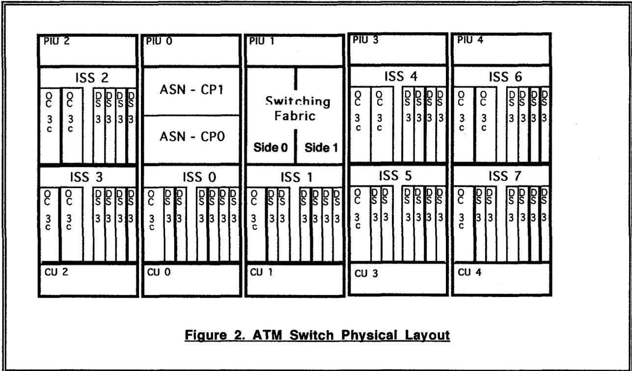
**Figure 2. ATM Switch Physical Layout**
