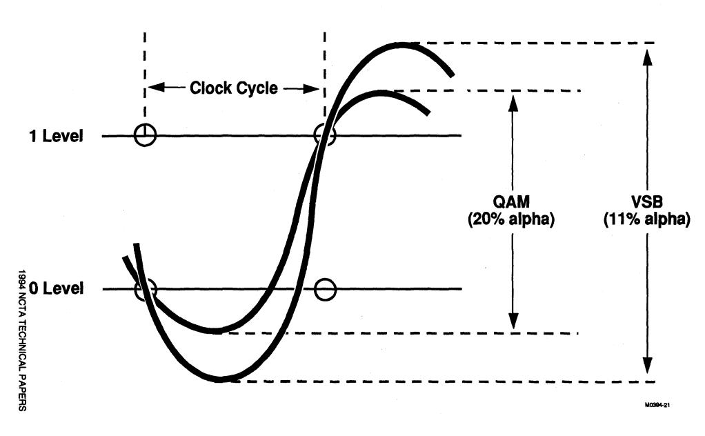
Figure 4 Overshoot for VSB (11% alpha) vs. QAM (20% alpha) with resulting 1.2 dB difference in peak power
