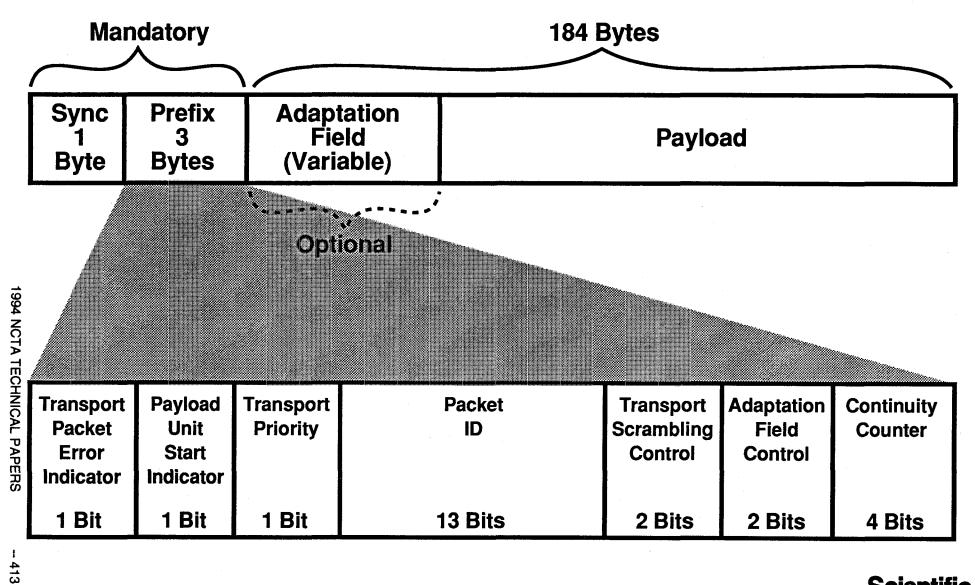
Figure 2 MPEG-2 Transport Packet Format
