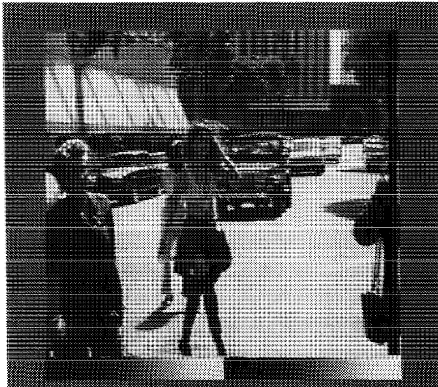
Picture with CSO and Thermal Noise (C/N = 35 db)
