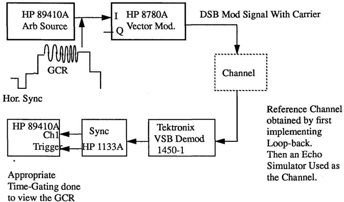
Fig. 1: Laboratory Setup Used for Channel Measurement.
