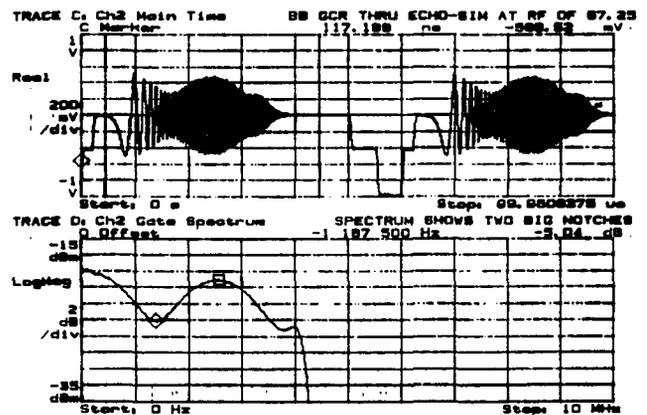
Fig. 5: GCR With a 10 dB Echo at 420 nsec.
