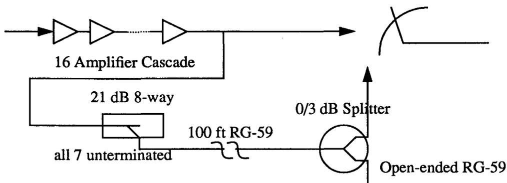
Fig. 12: Channel Setup for CATV Measurement
