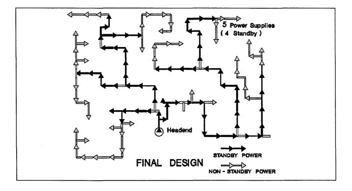
installed on the sub trunk legs. Four 15 ampere standby power supplies were then installed on the "main" trunk, and 30% of the existing power supplies were moved.
