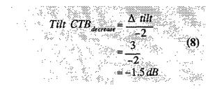
The total amplifier CTB change is the sum of the effects of the channel loading increase (2), the output level increase (5), the fiber link performance degradation (6), the reduction in RF amplifier cascade (7), and the increase in amplifier output tilt (8):
