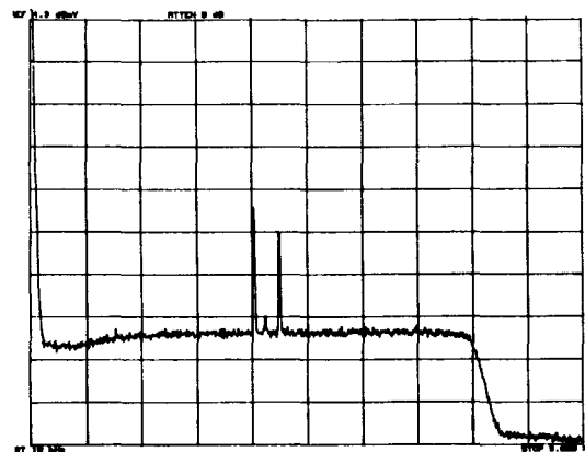
FIGURE 4. Fixed Frequency Modulator Baseband Noise Spectrum. Start: 10kHz Stop: 5MHz BW: 10kHz Ref: 4.3 dBmv 5dB/div
