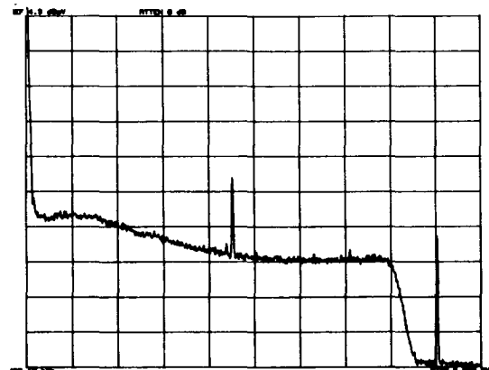
FIGURE 5c. Baseband Noise Spectrum Start: 10kHz Stop: 5MHz BW: 10kHz Ref: 4.3dBm 5dB/div
