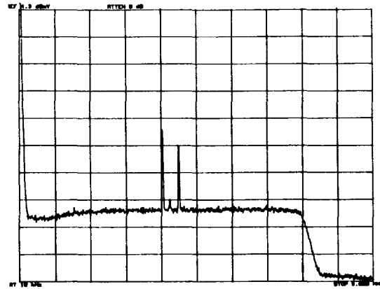
FIGURE 4. Fixed Frequency Modulator Baseband Noise Spectrum. Start: 10kHz Stop: 5MHz BW: 10kHz Ref: 4.3 dBm 5dB/div
