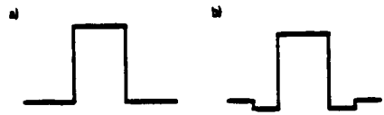
Figure 1. a. Standard step index profile (simple step index or matched cladding) b. Step index profile with reduced refractive index in the cladding (depressed cladding)
