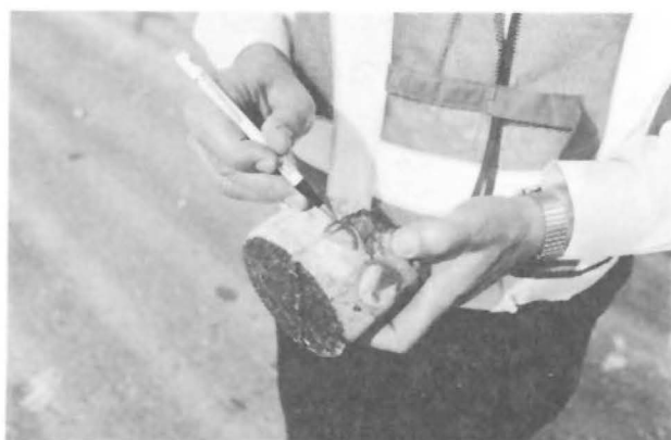
Fig. 5 - Core sample from above repaired highway pavement shows good bonding at surface and PERCOL penetration up to 2 1/2 inches deep.
