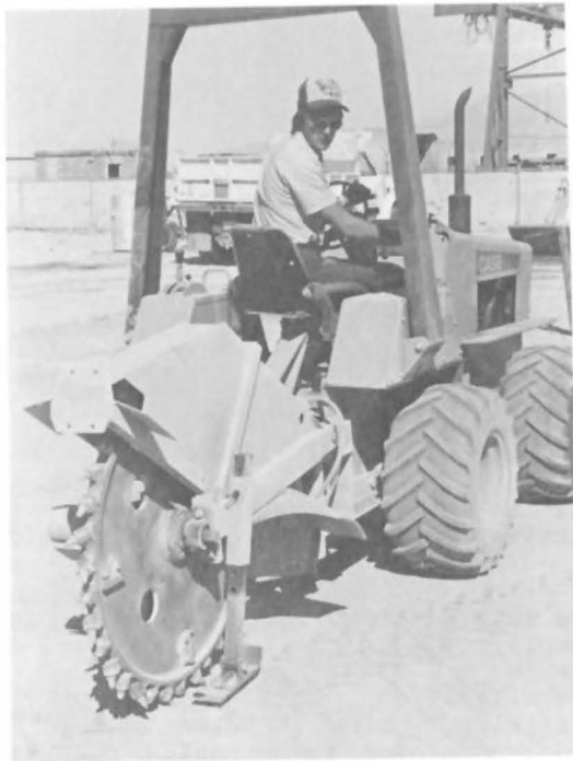
Fig. 14 - 36-inch carbide-tipped Case rock saw used to create 2 3/4 X 6 inch trench in pavement.
