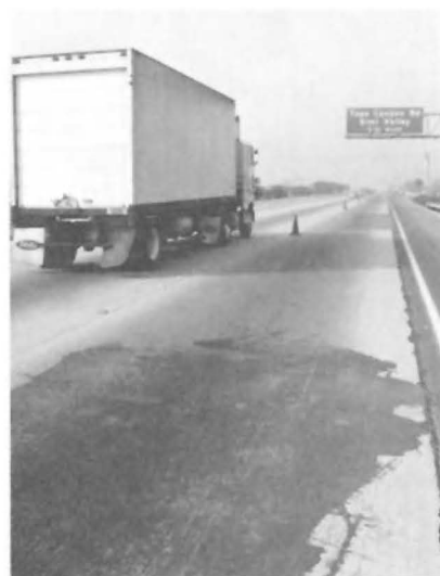
Fig. 4 - Caltrans PERCOL test on Highway 118, which carries average daily traffic load of 75,000 vehicles in each direction.
