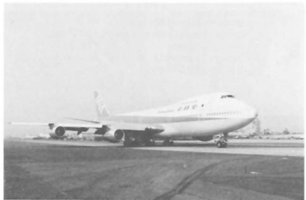
Fig. 9 - A 1200-ton aircraft taxis over the PERCOL-repaired runway.
