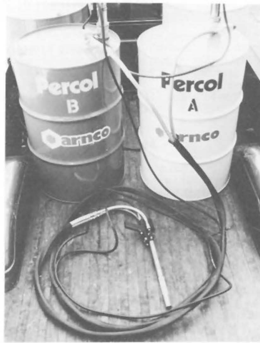
Fig. 1 - Simple equipment is used to pump liquid polyurethane "A" and "B" components from a pair of drums through a static mixer and nozzle.
