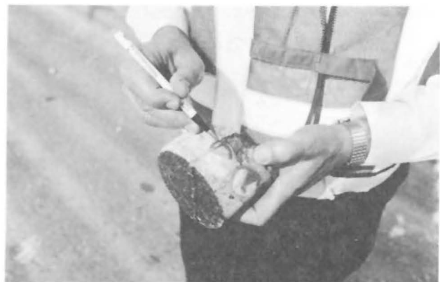
Fig. 5 - Core sample from above repaired highway pavement shows good bonding at surface and PERCOL penetration up to 2 1/2 inches deep.
