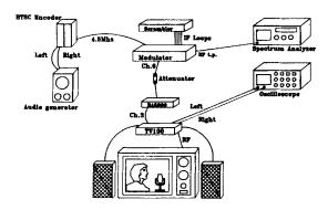
Equipment set-up and calibration was performed with a 1 Khz tone feeding the left and right channels of the BTSC generator. This enabled us to make an accurate determination of the input and output levels at each point in the system without regard for variations in program content. All equipment was calibrated to assure proper operation at all points.
