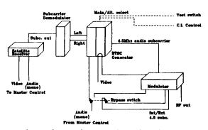
Connections when using a subcarrier demodulator are similar to the VideoCipher II connections except for the source of the left and right audio signals.
