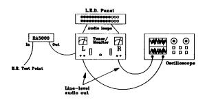
Output signal from a test converter is fed to the stereo receiver. High-impedance line-level audio output is routed to the LED display and to the oscilloscope. Modulation levels of both the left and right channels can be adjusted very accurately by observing the LED display. The oscilloscope is used for checks of separation and any scrambling components that may be present.
