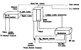
Stereo left and right audio is fed from the VideoCipher II directly to the BTSC generator. Program video and mono audio are routed through Master Control. Video is looped through the BTSC generator and terminated at the modulator.
