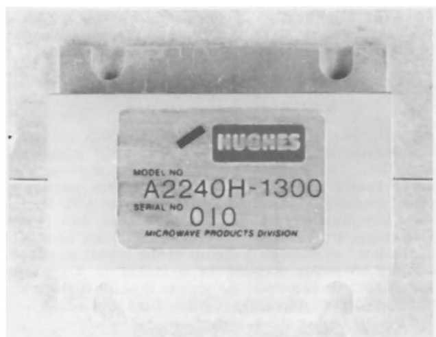
Figure 1 Ku-Band FET chip with 4-watt IMFET package.
