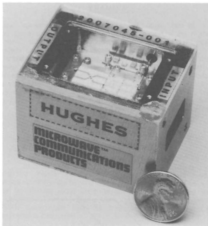
Fig. 4. Balanced LNA design implementation.
