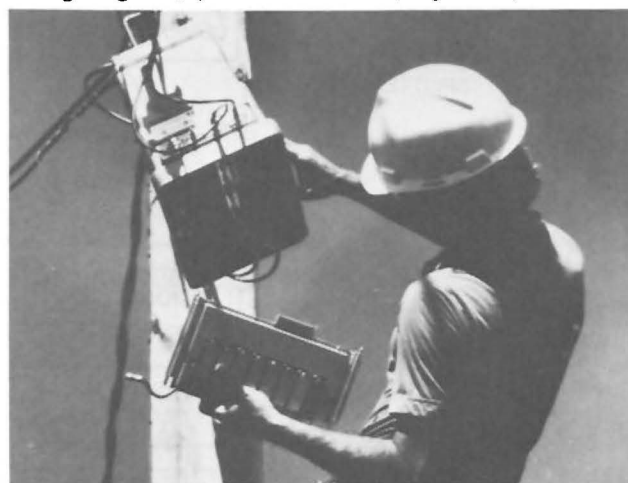
Fig. 1 OTAS Subscriber Terminal Each terminal has the ability to control seven (7) premium tiers plus basic on/off service per subscriber.
