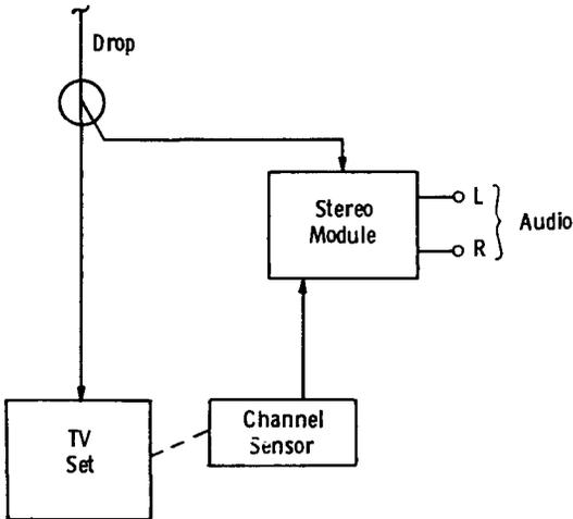
Figure 2. Stereo Module can be auto-tuned by sensing TV channel directly.
