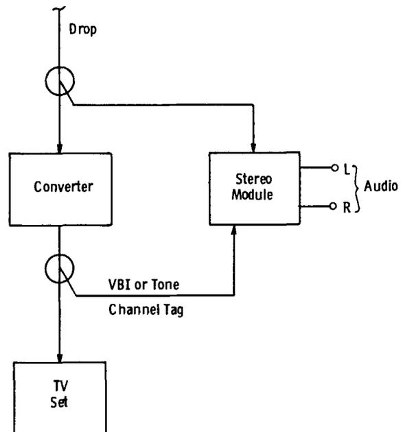
Figure 1. Stereo Module can be auto-tuned by VBI or tone 'tag' passed through converter.
