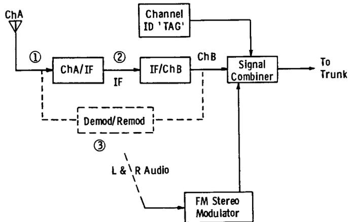
Figure 5. Full complement of equipment for modified headend.
