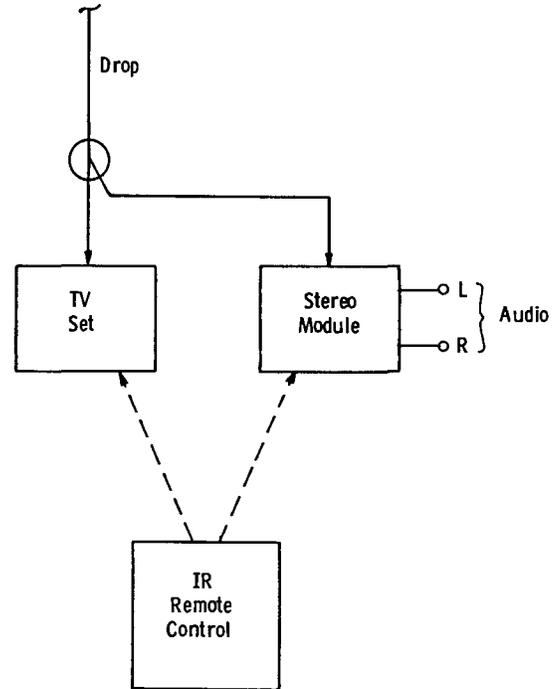
Figure 3. IR remote control tunes both TV and Stereo Module, and can offer remote-control volume.
