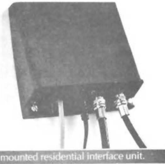
Wall mounted residential interface unit.
