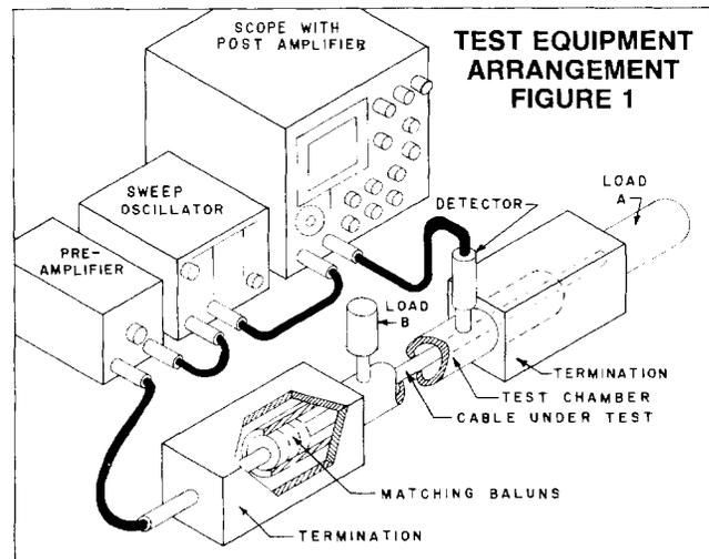
connected to the outer system by coaxial terminals. The rectangular termination on the ends of the chamber have ferrite toroids surrounding the test sample. These toroids minimize current flow along the shield of the test specimen to the end of the rectangular termination where the shield of the specimen is grounded. These rectangular terminations form "baluns" creating a high impedance allowing the load B and
