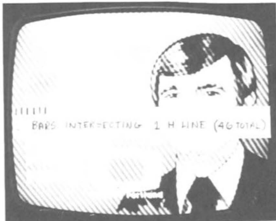
Figure 7 Count the Bars on one H Line in Center of Screen (1 MHz Intermod)
