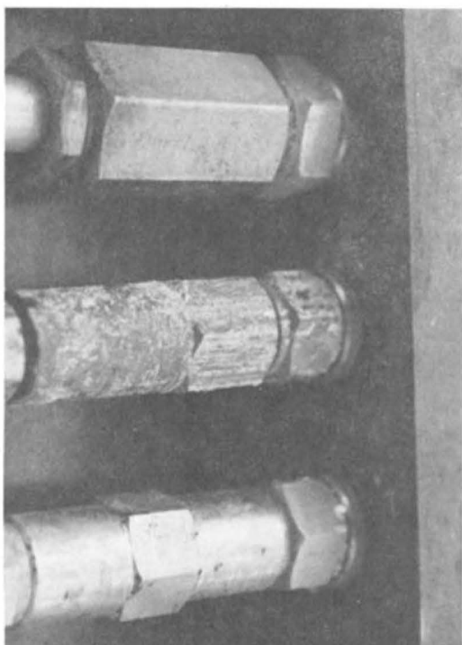
Figure 15. Appearance of three of the cable connectors after 90 days of high humidity/condensation testing. Top: 6262-T9 with chromate conversion coating. Center: 2011-T3 with no coating. Bottom: Unspecified aluminum alloy with bright tin plating [26].
