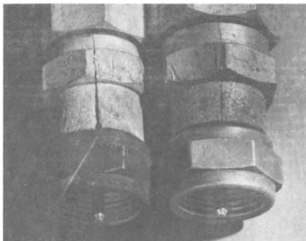
Figure 11. Photograph of two of the connectors removed from field installations near the seacoast after failing from stress-corrosion cracking. The cracks shown penetrate completely through the walls of the segments [26].
