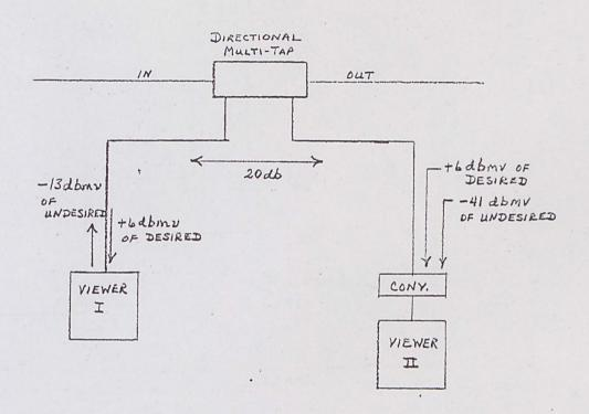
Viewer 1 does not have a converter and is tuned to Channel 5 using TV Receiver Set C which has an oscillator leakage of -13 dbmv. Viewer 2 is tuned to Channel A. Both lines are delivering +6 dbmv of desired signal.
