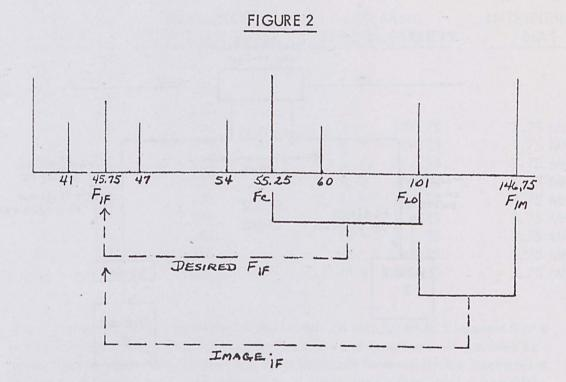
Here we see desired Channel 2 at 55.25 MHz beating with the local oscillator signal at 101 MHz to produce IF at 45.75. Also observe that a signal at 146.75 can beat with the local oscillator to produce the desired IF signal. The 146.75 MHz frequency is referred to as Channel 2's image. Its presence into the receiver's IF is limited by the tuner's image rejection capability. Image rejection typically runs as follows:
