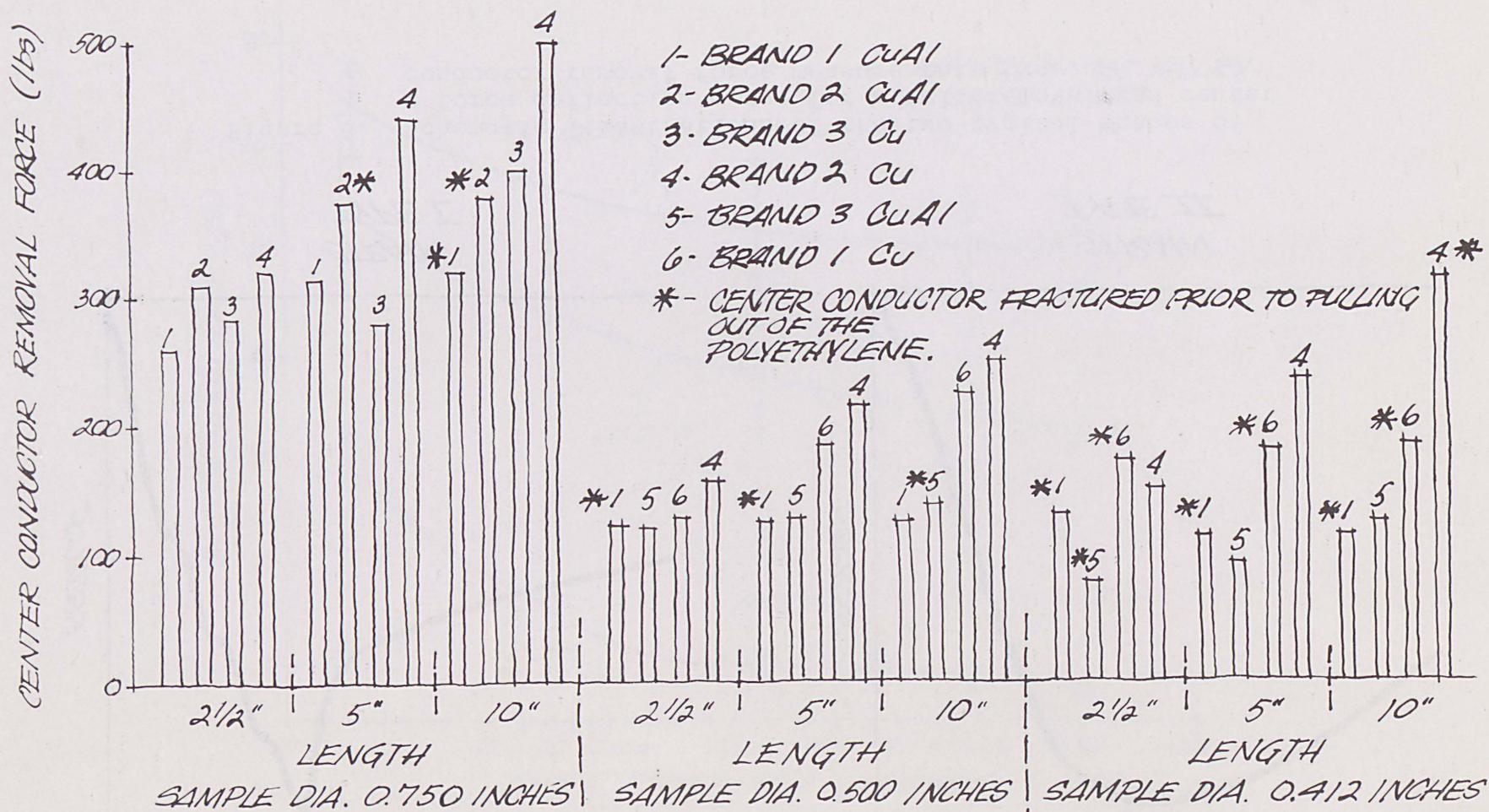
Figure 5. Center conductor removal forces for various manufacturers, sample lengths, cable diameters and center conductor materials.
