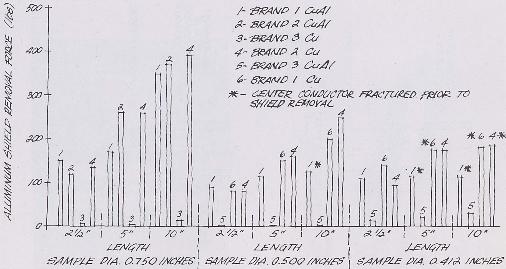
Figure 4. Aluminum shield removal forces for various manufacturers, sample lengths, cable diameters and center conductor materials.
