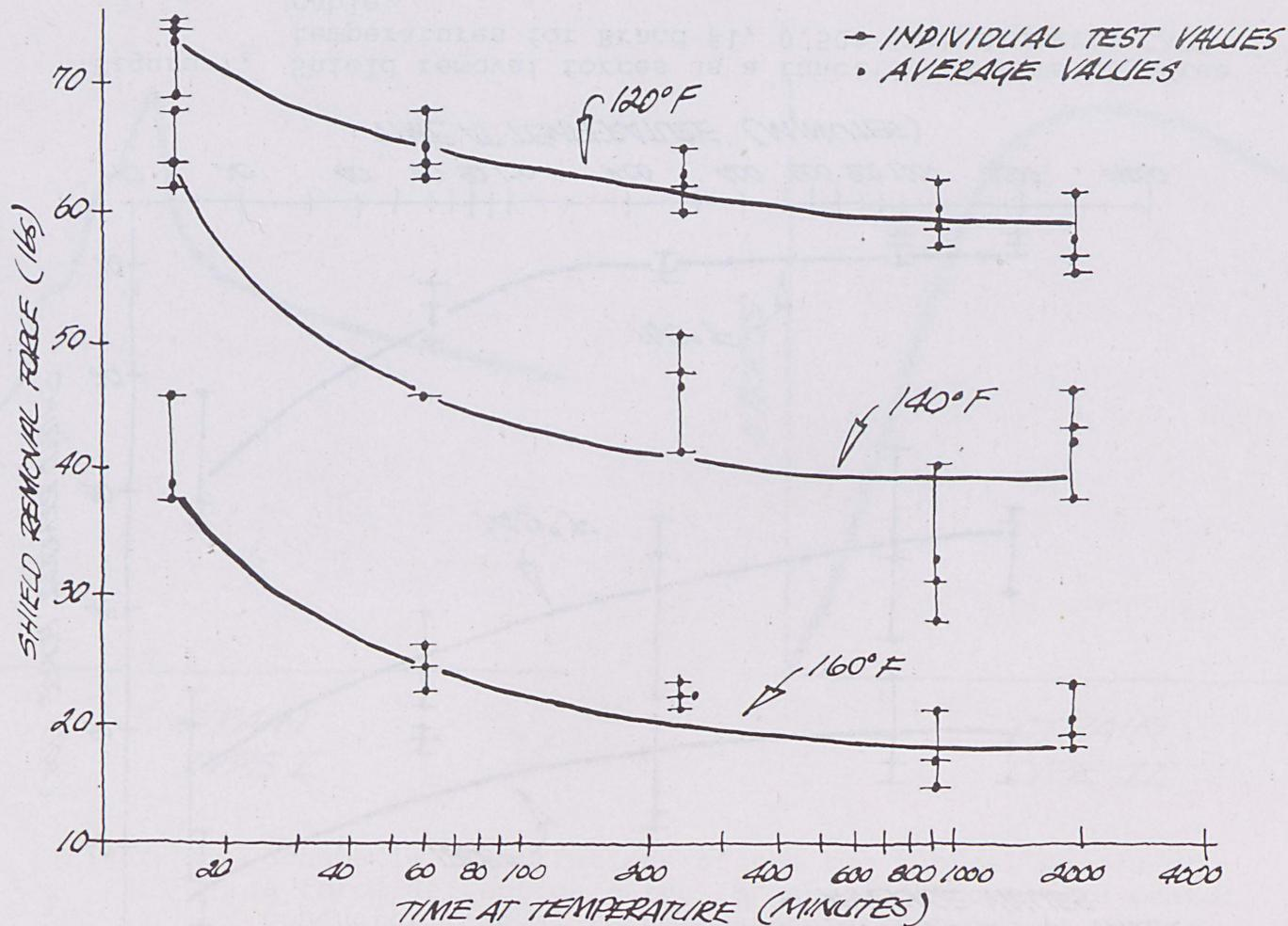
Figure 8. Shield removal force as a function of time at three temperatures for Brand #1 0.750 inch diameter CATV cable.
