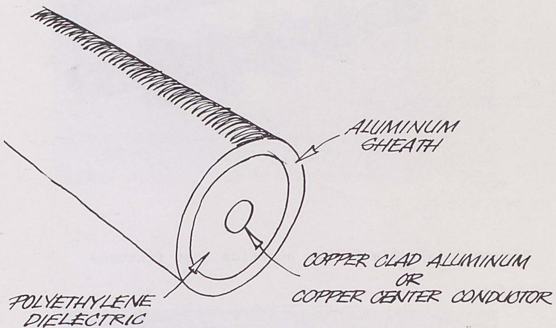
Figure 1. Schematic diagram of an aluminum shielded CATV cable with a foamed polyethylene dielectric.
