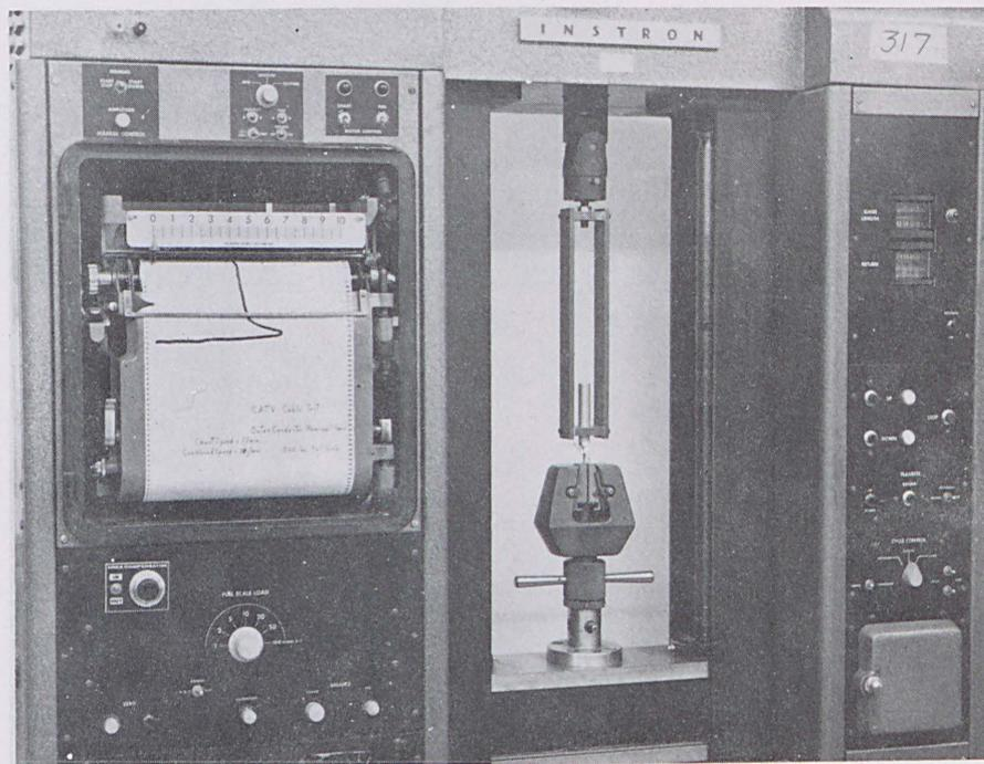
Figure 2 (b) Test fixture and specimen in position on Instron Tensile Testing Machine
