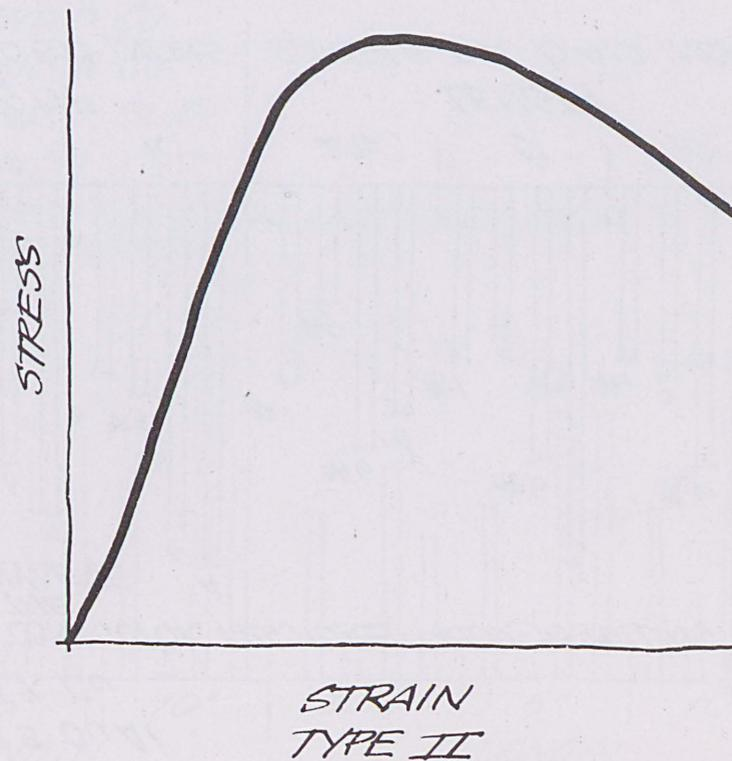
Figure 6. Schematic illustrations of the two typical shapes of a force deflection curve for shield removal and center conductor removal force measurements type.
