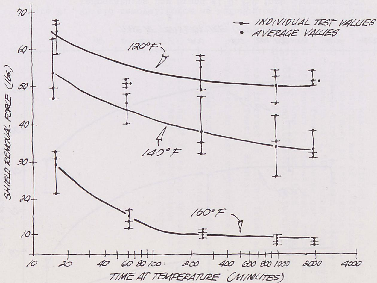
Figure 7. Shield removal forces as a function of time at three temperatures for Brand #1, 0.500 inch diameter CATV cable.
