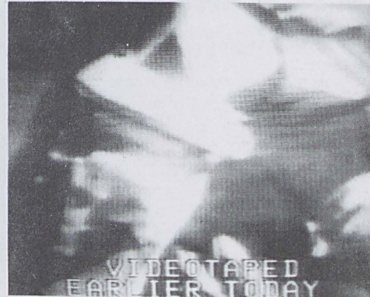
Fig. 17. TV picture with 40 dB down interfering signal.
