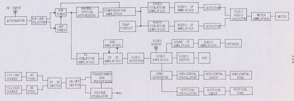
FIGURE 1 FIELD STRENGTH METER MODE FIELD STRENGTH MONITOR
