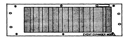
Event Expander Chasses, Model EE-1000, are available to accommodate additional Program Cards when the number of switching events designated to a given output exceeds the card slot capacity of 15 provided to allow a Program Card to be delegated to operate with either output in either of two associated OC-1000 Output Control Chasses. The Event Expander Chassis is a passive device, and may be connected as necessary to extend system event capacity.
