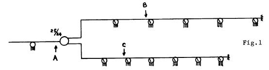
Signals arrive at the cable split with  $+25 \, \mathrm{dBmV}$  at ch 13 and  $+24 \, \mathrm{dBmV}$  at ch2. By merely splitting the signal amplifiers are required at point B and point C.
