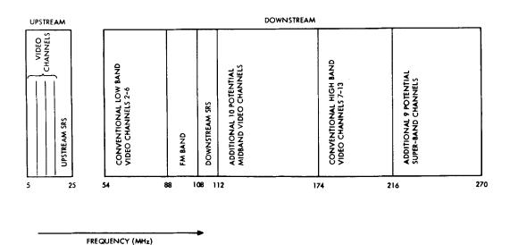
Figure 5. Cable Spectrum Allocation
