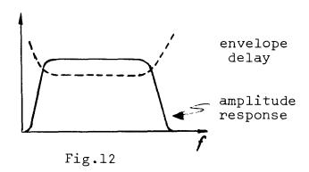
Delay measurements also require very good impedance matching all around; because mismatch causes reflections with resulting ghosts, and ghosts are a delay phenomena also.
