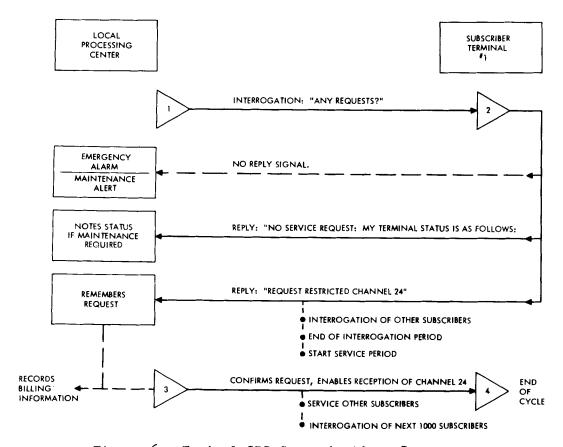
Figure 6. Typical SRS Communications Sequence
