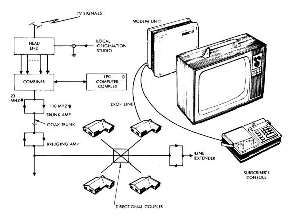
Figure 1. Overall CATV Two-Way System
