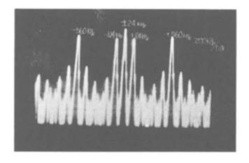
Photo 8 TRANSMISSION SPECTRUM AFTER 10 CASCADED TRUNK AMPLIFIERS
