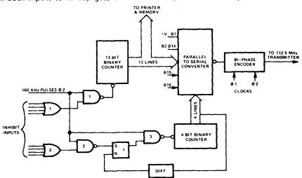
Figure 14 Address Generator & Multiplexer
