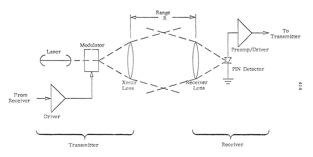
FIGURE 2. SCHEMATIC FOR ONE CASCADE LINK ELEMENT FOR CATV
