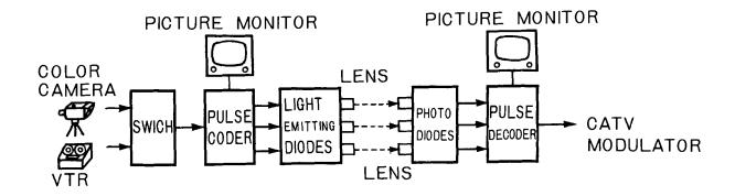
Fig. 3 OPTICAL COMMUNICATION LINK
