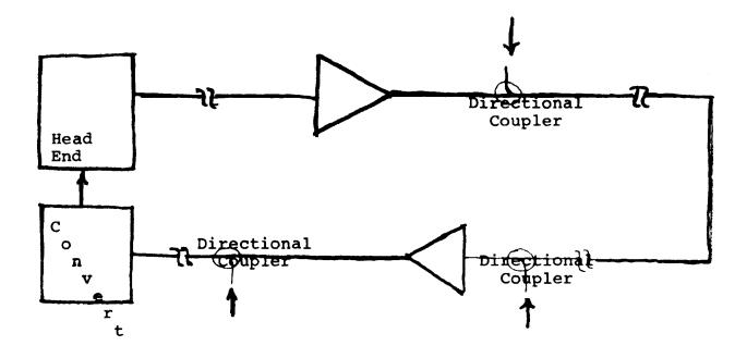
Figure 1 Closed Loop System
