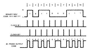
Figure 6 Bi-Phase Encoder Timing Diagram
