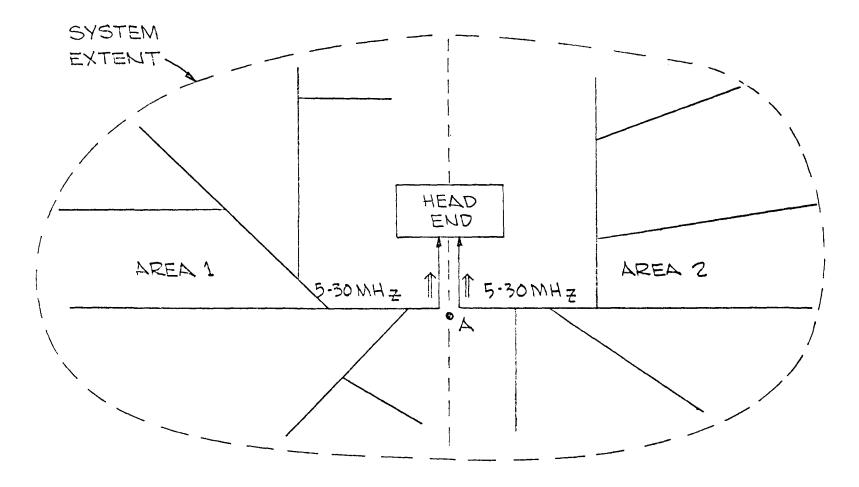
If two return cables are employed from point "A" to the Head End, and the areas are approximately equal, the C/N will be 3 dB better than if the return cables were combined at "A".
