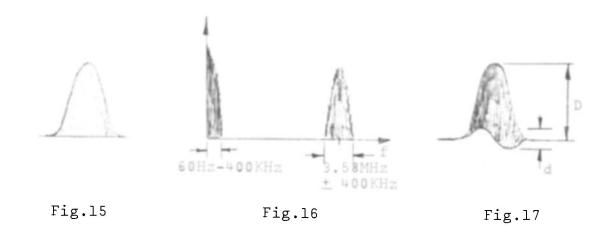
The base line of this pulse gets distorted when the signal is passed through a device with chroma delay. It is possible to determine the delay by measuring pulse height (as referenced to the bar signal level) and the base line excursion using graphs or formulas.
