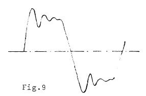
The output is non-symmetrical with a very pronounced ringing. As a further example let us shift the 3rd harmonic by 30°, the 5th by 60° and the 7th by 90°:
