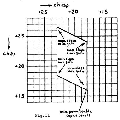
The internal slope control can reduce the gain at Ch 2 by 8dB. Therefore any point on the vertical line between 18/16 and 18/24 can be amplified to the desired output 40/36, by proper adjustment of the slope control. Similarly the gain control line between 18/16 and 23/18.5 indicates the levels which can be accommodated with the gain control.
