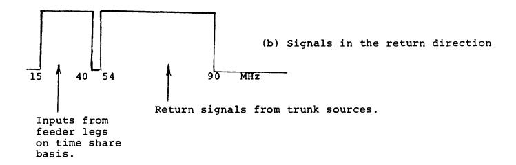
Figure 5 Band Pass of Dual Cable Bi-Directional System
