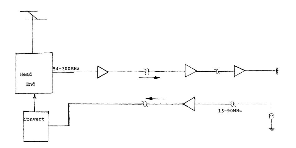
Figure 4 Dual Cable Bi-Directional System
