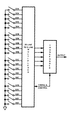
Figure 19 Using the Transponder for Sensing 20 Independent Switch Inputs
