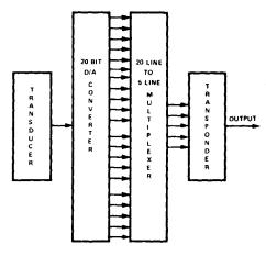
Figure 20 Using the Transponder For Monitoring One Input Parameter For 1,048,576 Discrete Measurement Levels
