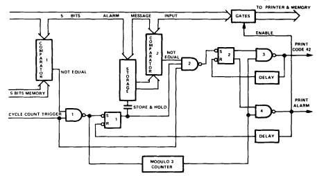
Figure 16 Alarm Comparator
