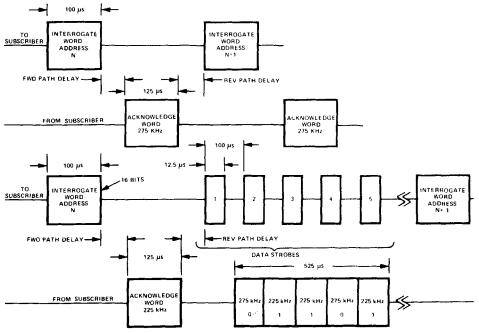
Figure 11 System Timing Diagram
