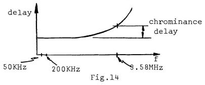
Chroma delay is one of the most visible effects of envelope delay and methods to measure it rapidly have been developed. The 20T pulse has gained wide acceptance for measuring chroma delay; it is a low frequency pulse modulated with 3.58 MHz color subcarrier signal. Its shape and frequency components are pictured below:
