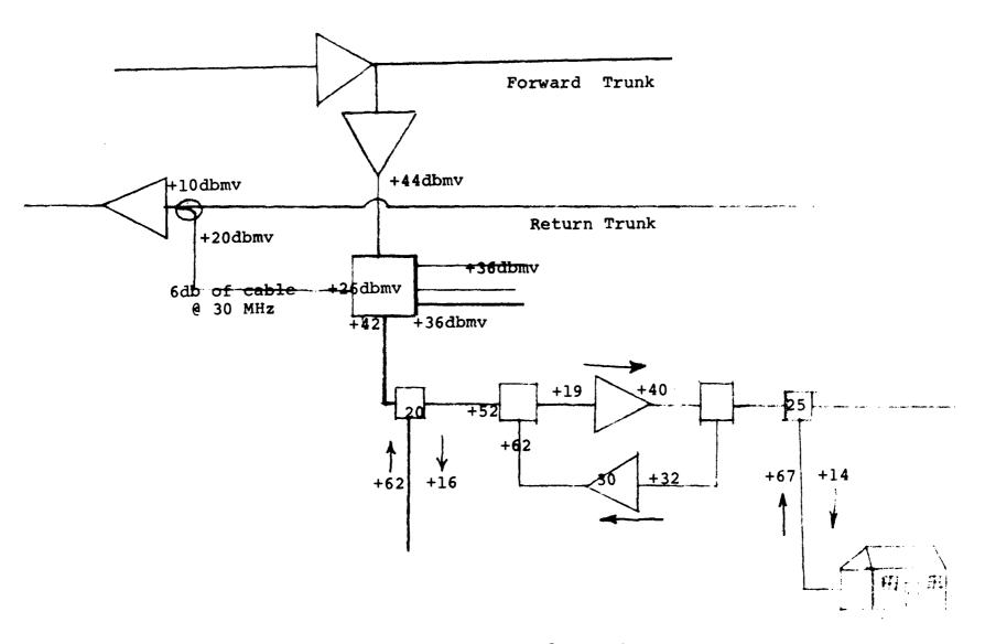
Figure 6 Bi- Directional Feeder System
