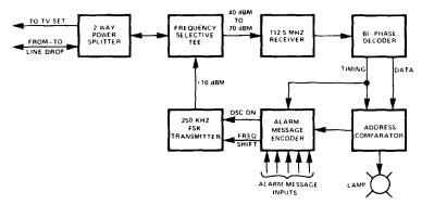
Figure 10 Block Diagram Subscriber Station
