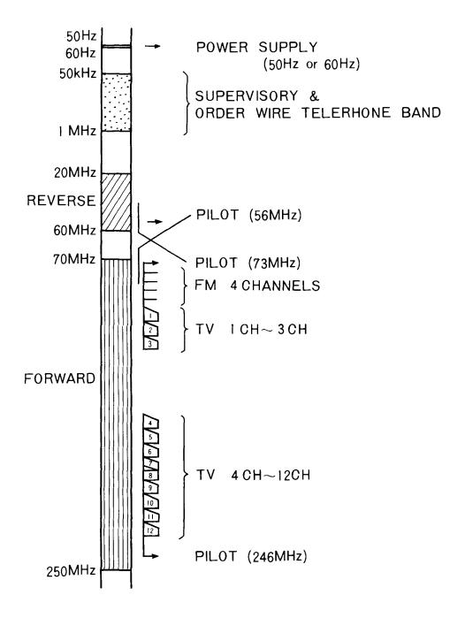
Fig. 2 FREQUENCY ALLOCATIN OF BI-DIRECTIONAL CATV SYSTEM
