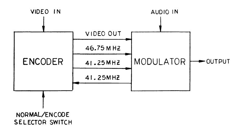
FIGURE 2-INTERCONNECTIONS BETWEEN ENCODER & MODULATOR
