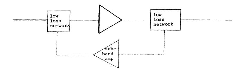
Figure 3 Single Cable System using loss filter networks
