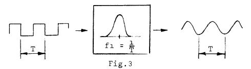
We also get a sinewave output if we feed the square wave through a filter with a bandpass for three times the fundamental frequency.
