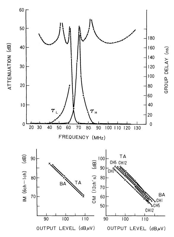
Fig.11 MEASURED INTER & CROSS MODULATION VERSUS OUTPUT LEVELS FOR TRUNK & BRIDGE AMPLIFIER.
