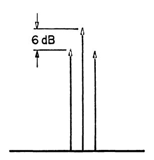
SPECTRAL LINES OF A CARRIER 100% MODULATED WITH A 15.75 KHz SIGNAL
