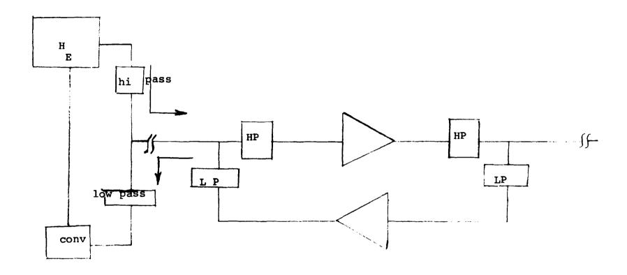
Figure 2 Single Cable System using standard diplexing filters
