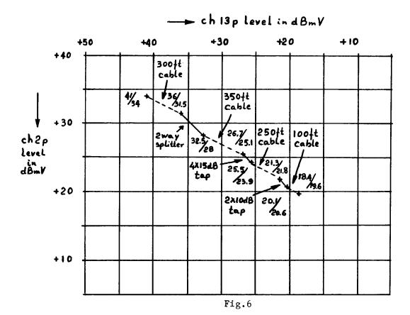
The graph can contain more information. Figure 7 shows the 2 way  $10\,\mathrm{dB}$  tap again; the horizontal dimension of that square represents the through loss at ch 13p; the vertical dimension represents the through loss at ch 2p.
