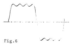
The result is not a very good square wave since one should also add the 9th, 11th and all other odd harmonics to make a true square wave. It should also be noted that a square wave does not contain any even, such as 2nd harmonics. The principle, however, holds.
