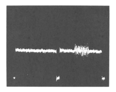
Inserted noise is much greater than noise on signal
