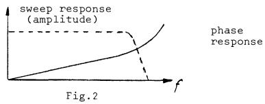
To be more specific we should label the sweep response amplitude response; after all the familiar sweep generator setup measures the amplitude versus frequency characteristic. The phase characteristic is seldom measured, but we believe this will become more common place in the future, particularly for single channel devices.
