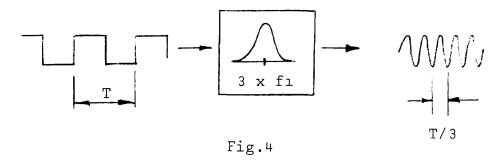
The same will happen if we use a filter for 5 times the fundamental, also for 7 times, 9 times, etc.
