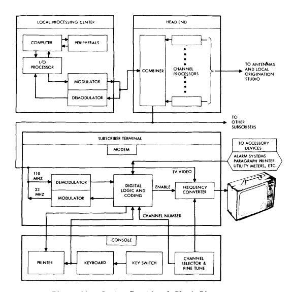
Figure 14. System Functional Block Diagram
