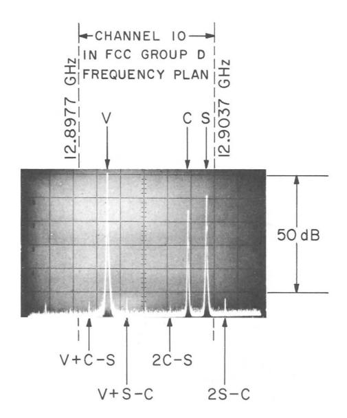
Fig. 8. MEASURED IN-BAND THIRD-ORDER INTERMODULATION PRODUCT AMPLITUDES OF CHANNEL 10 CARS-BAND TRANSMITTER
