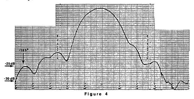
Figure 4 illustrates the need for F/B ratio specifications and radiation pattern comparison. The manufacturer's specifications stated 30 dB protection from the back. The radiation pattern indicates that indeed the diamond quad
