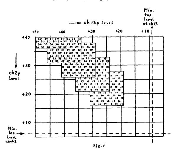
Since operators use different types of drop-cable and have different ideas as to what the tap levels should be, the area information and minimum required tap levels is printed on a transparent overlay and can be shifted to any operator's heart's content.
