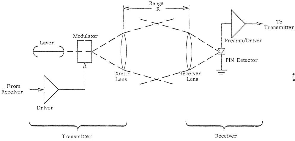
SCHEMATIC FOR ONE CASCADE LINK ELEMENT FOR CATV FIGURE 2.
