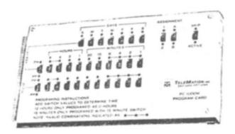
The output from the Program Card can be assigned to any of four different channels, depending on the placement of the assignment switches directs the output of the assigned output control chassis or OC-1000.
