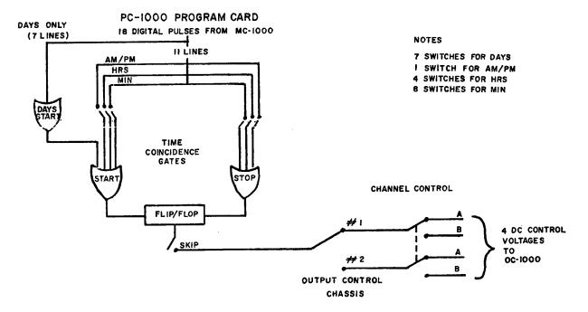
The PC-1000M Program Card controls one complete switching event from start to stop. This card also permits selection of day or days of the week that the switching event will occur. The 18 digital pulses from the Master Clock are routed to the days-only gate through the selected day switch. Eleven lines are then routed to the start time coincidence gates through the selector switches for AM or PM, hour, minutes switches. If one of the programmed days is the same as the day
