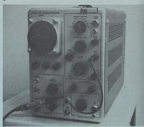
Actually, it is a high quality oscilloscope that has a calibrated time base and a vertical amplifier with a pass of DC to 10 megaHertz. This is a limiting factor cause no determination can be made concerning the quency characteristics of the information displayed to megaHertz.
