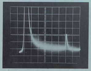
This is the same cable with the end still terminated with the gain of the scope at maximum and we begin to see some of the physical defects in the cable. NEXT SLIDE PLEASE (#13)
