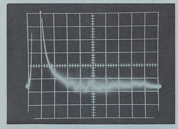
This is the same cable with the time base of the scope changed to .2 microseconds per division and the gain increased to .05 volts per division. At this setting of the scope, each division is worth about 80 feet of cable and you can see it is well riddled with reflections.
