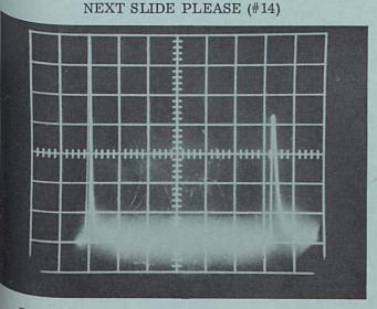
Scale is 1 microsecond per cm., or 400 feet per division. This is about 2500 feet of cable with two pressure taps and an amplifier at the end of this 2400 feet. This end looks open but again we are not making conclusions as to frequency.
