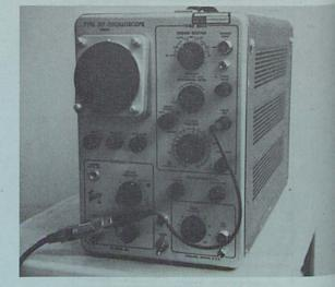
Actually, it is a high quality oscilloscope that has a calibrated time base and a vertical amplifier with a pass of DC to 10 megaHertz. This is a limiting factor cause no determination can be made concerning the puency characteristics of the information displayed in 10 megaHertz.
