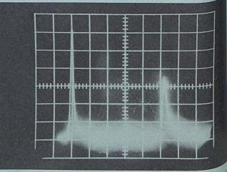
Here the scale is .5 microseconds per cm., or et pre to 200 feet per division. This is about 1050 feet of call 240 with a pressure tap and ending in a two-way splitter doesn't mean the splitter isn't good because, as I me earlier, we are limited to physical factors because d band width of the scope.
