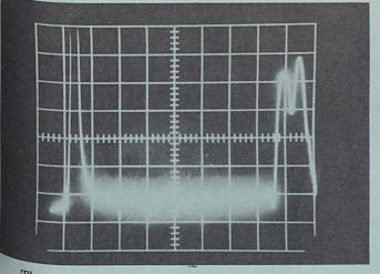
The scale here is .5 microseconds per cm., over <sup>7</sup> divisions or 1500 feet. This is about 1500 feet of <sup>cable</sup> with taps at 200 feet, 400 feet, 600 feet and <sup>Another</sup> splitter at the end. Probably one or both of <sup>the</sup> legs of the splitter are not properly terminated.
