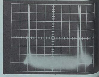
The scale here is 1 microsecond per cm., or ab 400 feet per division over 6 divisions equals about 25 feet. Here we see about 2500 feet of two types of cab The first 1400 feet is fairly new cable with a splice 1100 feet and another splice at 1400 feet. The remain is older cable that has been in the air for a number years.
