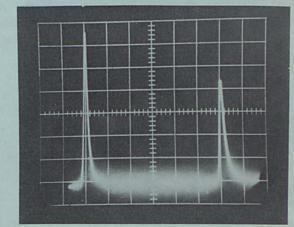
This slide shows about 1200 feet of foam cable with the end open. The scale horizontally is .5 microseconds per division, equal to 200 feet of cable - vertically is .1 volts per division.
