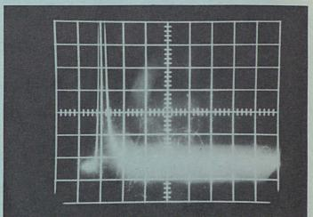
.5 microseconds per cm. Here is about 700 feet of feeder line that is pretty bad. If you were to cut into this piece you would probably find the outer conductor black and drops of water all through the foam.
