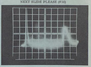
This is .5 microseconds per cm., with 200 feet per division. This is about 1200 feet of cable with two pressure taps and ending in a splitter. The termination of the legs of the splitter appears normal.
