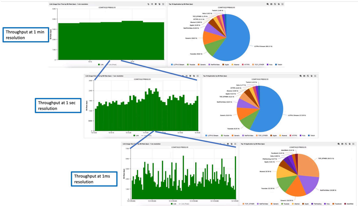
Figure 6- DOCSIS Serving Group Utilization Characteristics per Observation Time Windows (source: NetScout Packet Inspection Tool)
