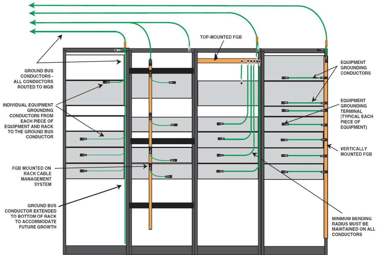
**Figure 2 – Acceptable Interior Grounding Methods - Network Equipment Racks**
