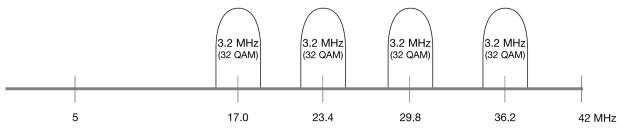
Figure 7 – Large Guard Bands Between Upstream Channels
