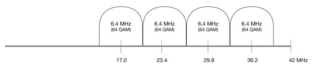
Figure 9 – Maximizing Upstream Capacity With Wide Upstream Channels and Small Guard Bands
