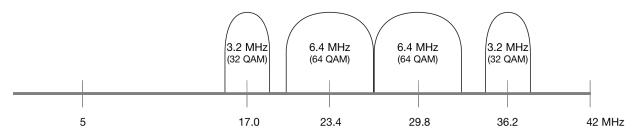
Figure 8 – Increasing Channel Width To Increase Upstream Capacity
