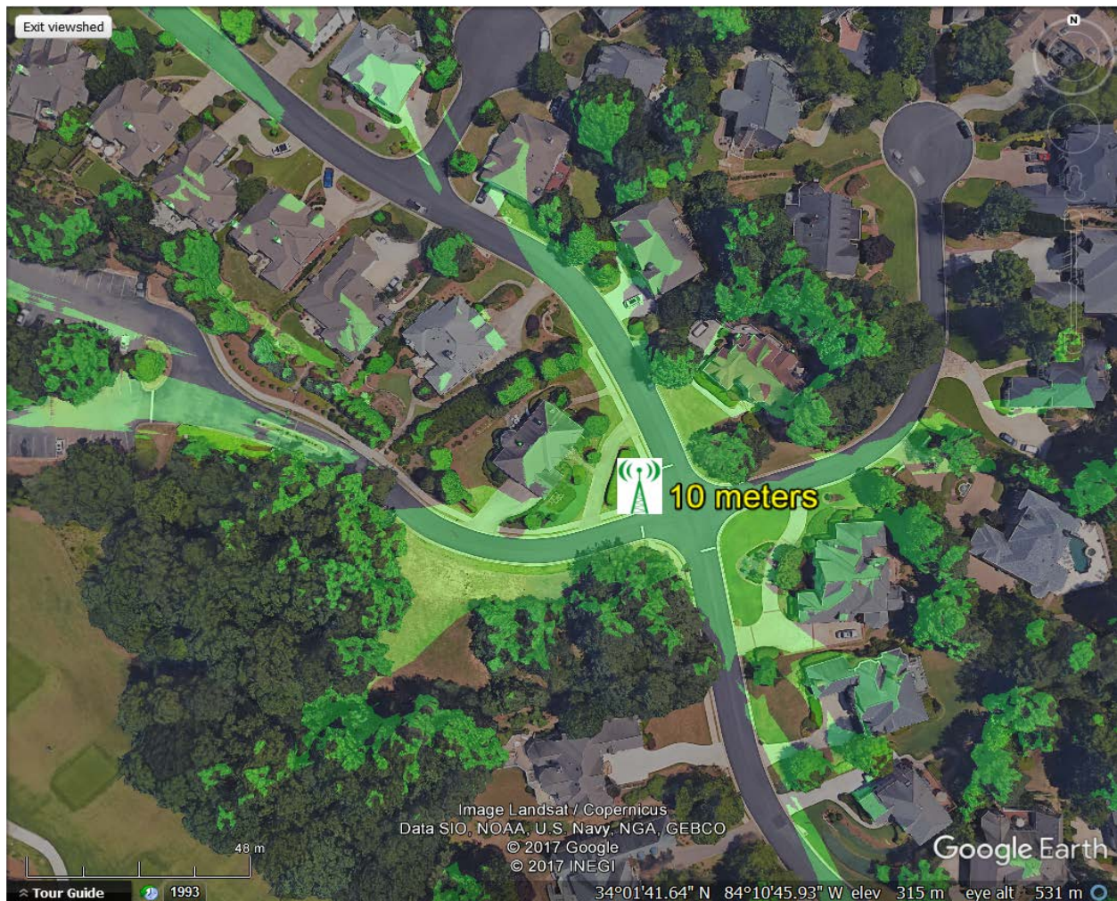
Figure 8 – LOS “Look” Mask from 10 Meter Mast (lime green shadow)
