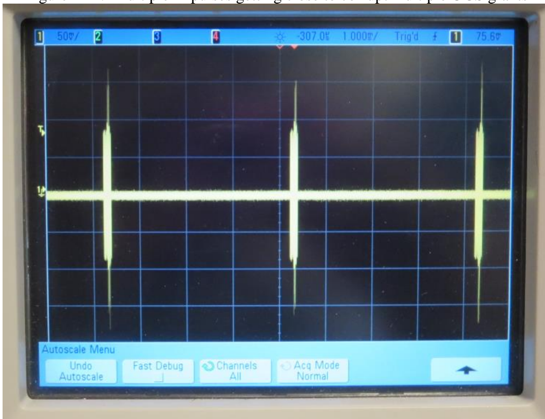
Figure 11B. Multiple impulses are corrupting multiple UGS grants. Note the signal & noise addition.
