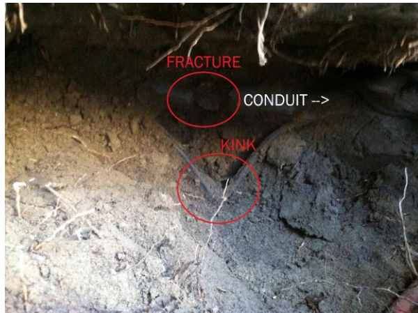
Figure 12. The kinked corroding cable causing the high second order distortion for location 3.
