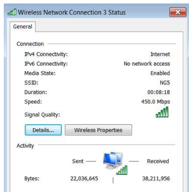
Fig. 12 3by3 AP and 3by3 STA reporting 450 Mbps modulation and coding scheme
