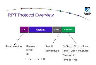
Central to RPT is the ability to enable switching and transport at the packet level. Packet level processing yields infinite granularity and maximizes transport bandwidth efficiency. Eliminating the need to map bandwidth into preconfigured circuits that are always the wrong size. RPT enables the provisioning of more services to more customers over the same cable backbone Transport bandwidth may be network. provisioned in exacting amounts with flexible burst capability.
