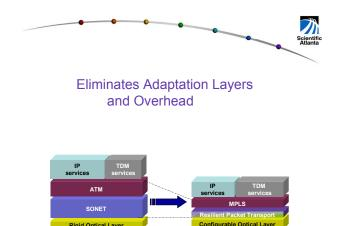
The RPT packet includes a 6 bytes RPT header and 4 bytes MPLS and contains all the necessary information to move the packet through the network. This is a very small tax relative to SONET and ATM for similar functionality.
