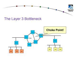
RPT eliminates the layer three bottleneck and expense by operating in Layer 2-1/2 and using the RPT header for pack destination information. As each packet traverses network, the RPT header determines if the packet should be dropped or passed. RPT enabled boxes will likely reduce network dependence on high capacity routers.
