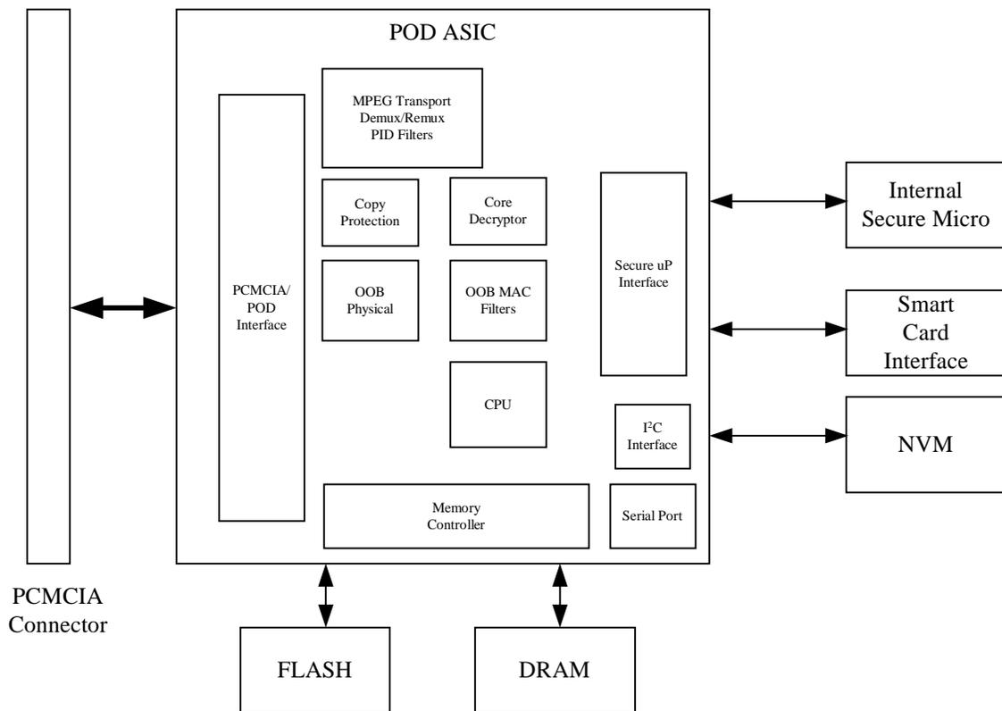
To fit the amount of functionality the POD specifications require into a small form factor such as Type II PCMCIA, considerable integration in silicon is called for. Thus, much of the major components in the POD block diagram above are found on an ASIC. This chip, of course, has interfaces to memory and other chips such as secure microprocessors to complete its mission.
