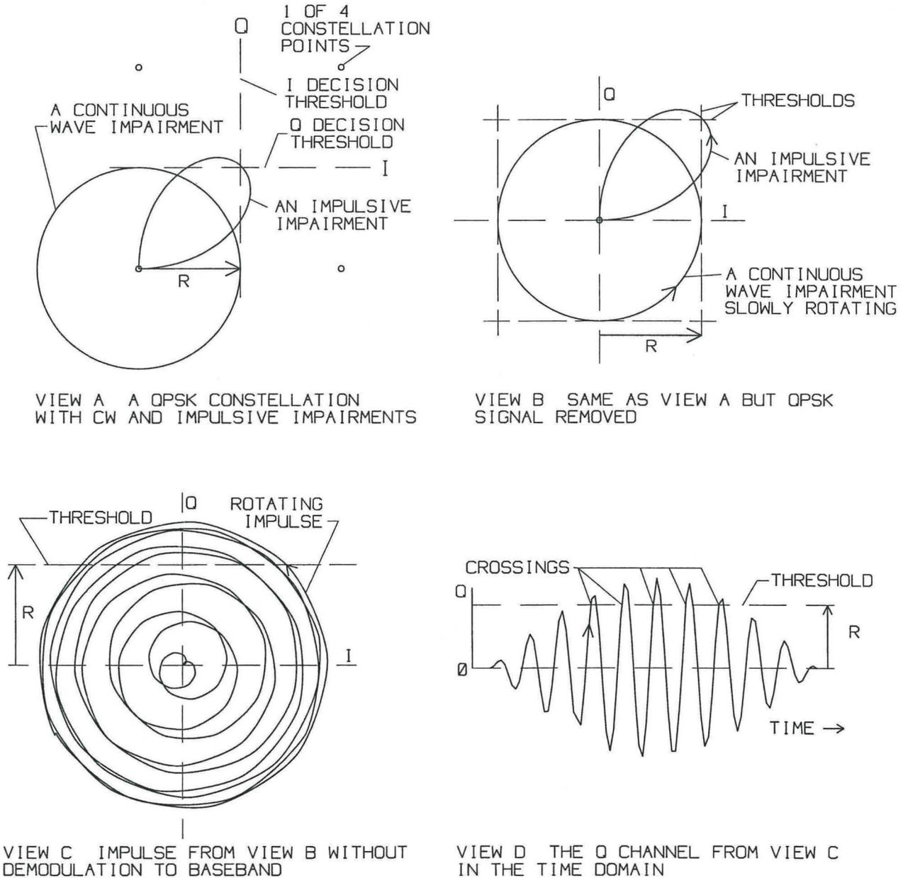
**Fig. 5 I-Q Diagrams Illustrating how impairments can be characterized with a bandpass filter and a totaling counter.**
