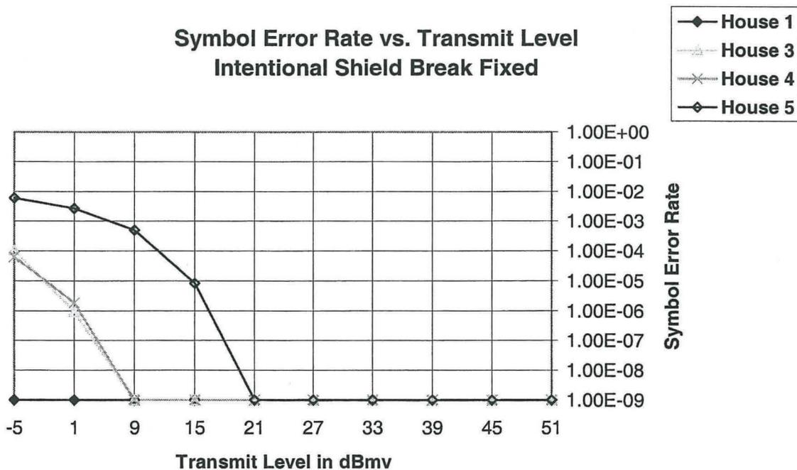
**Fig. 15** Required QPSK transmit level at a tap port for a given symbol error rate in the presence of burst noise generated on house's AC power wiring. The intentional shield break at the ground block is repaired.
