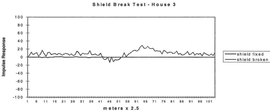
**Fig. 8 Long buried drop (142 ft.). Gross power =29.2dB broken, =4.4 dB unbroken
