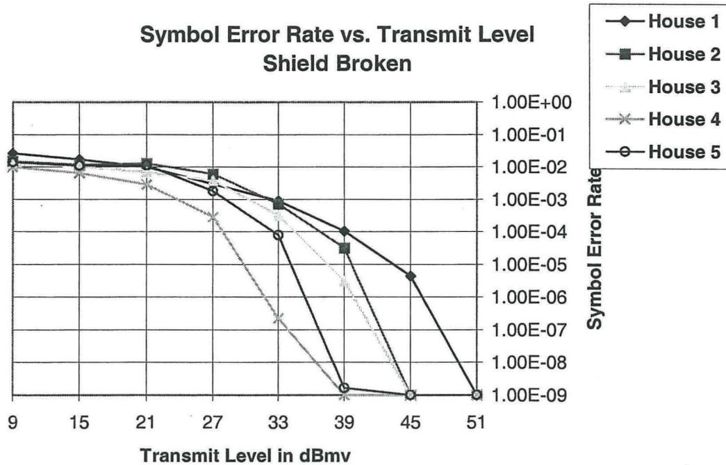
**Fig. 14** Required QPSK transmit level at a tap port for a given symbol error rate in the presence of burst noise generated on house's AC power wiring. Shield intentionally broken at the ground block.
