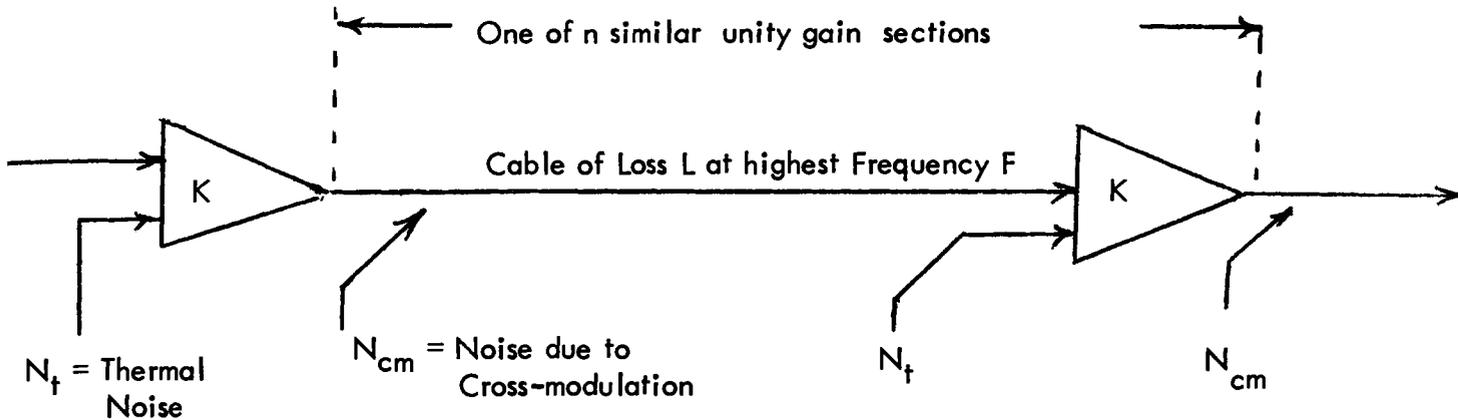
The preceding drawing shows one of n unity gain sections of a cable transmission system. Let the video signals be applied in a frequency division multiplex arrangement using a modulation system comparable to conventional broadcast standards. Let the cable loss for the highest frequency channel be L and the gain of the amplifier (including a built in cable equalizer) be K where
