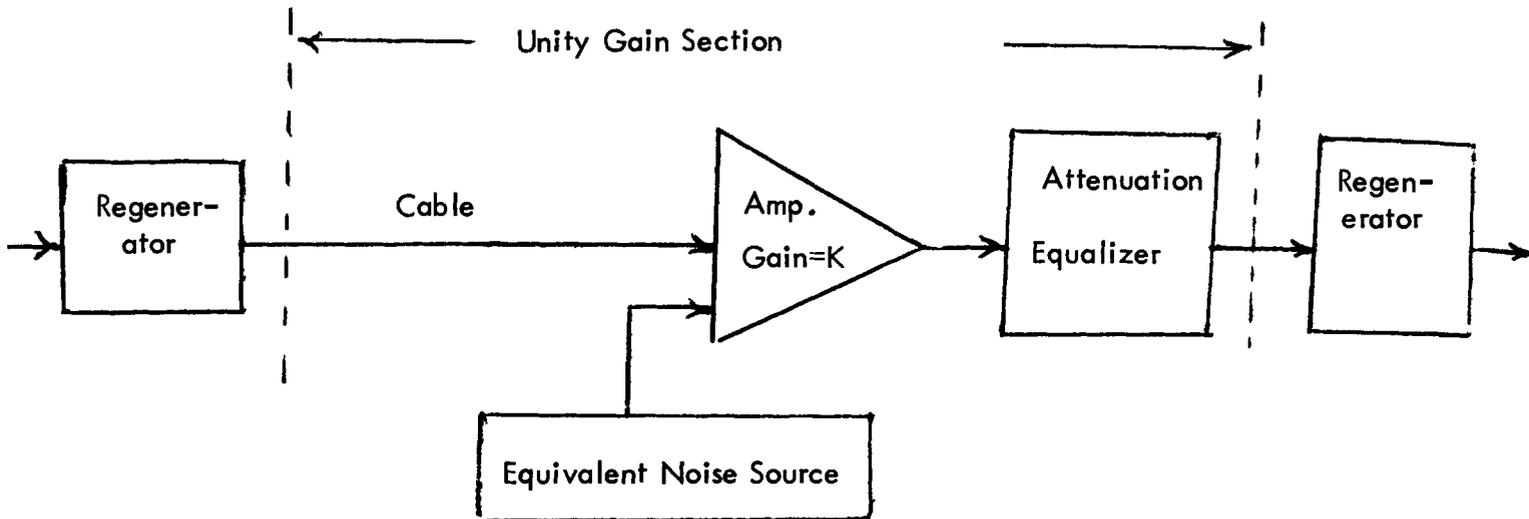
The preceding drawing shows a typical digital repeater section, with the regenerator driving the coaxial cable whose loss is given by:
