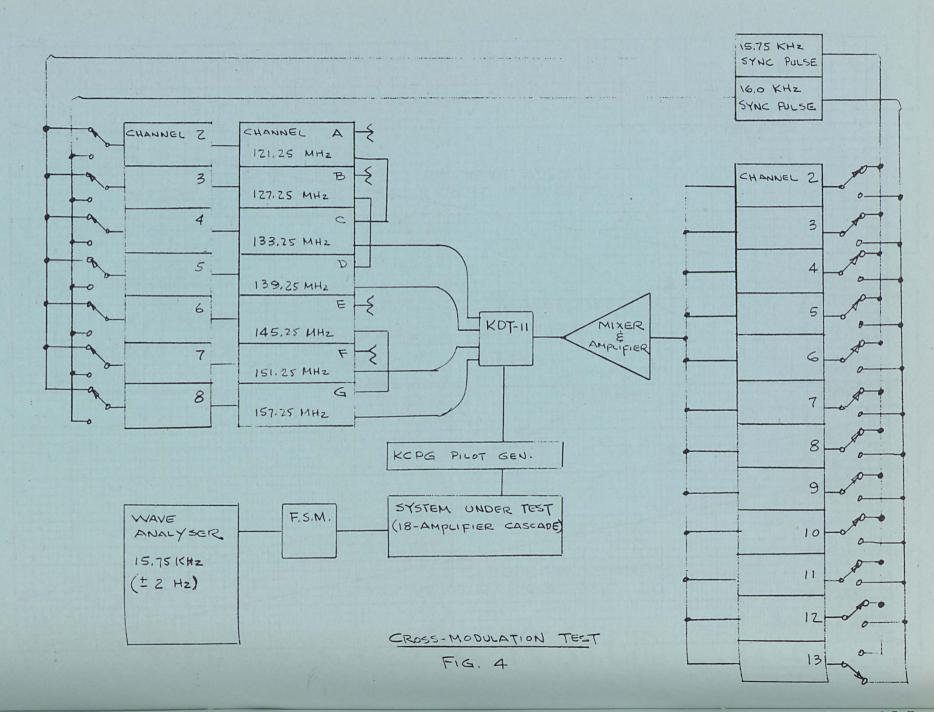
Single amplifier output level capability with a -57 dB cross-modulation indicated on all channels, minimum. The KAISER "White Screen Tester" (see Figure Nos. 1 & 2) is used in these tests.
